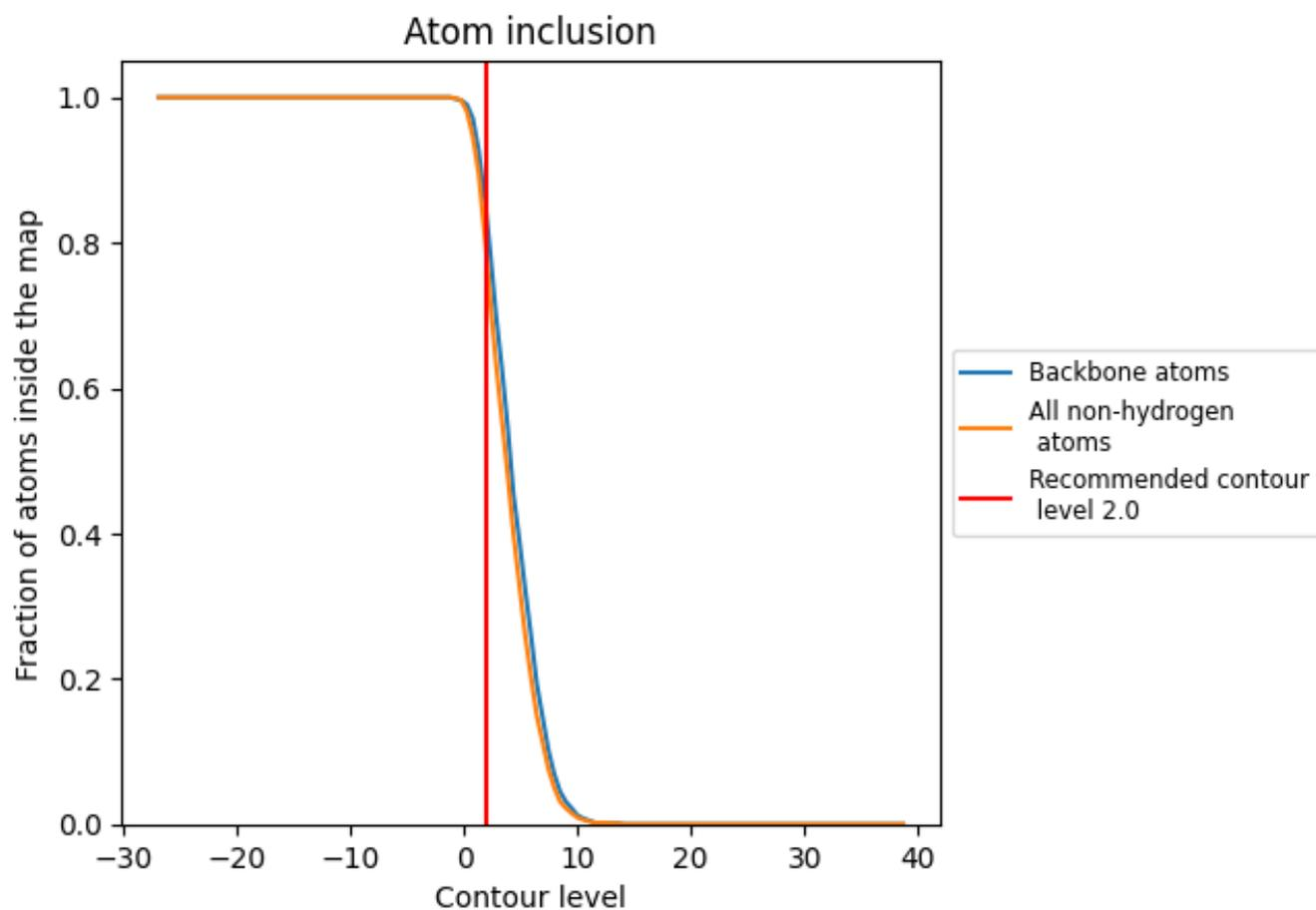
At the recommended contour level, 84% of all backbone atoms, 78% of all non-hydrogen atoms, are inside the map.
