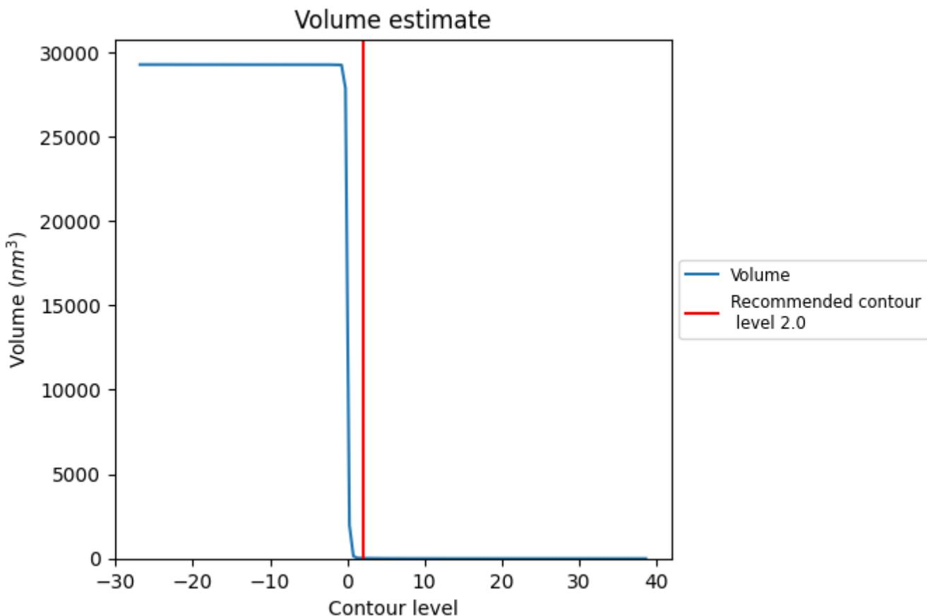
The volume at the recommended contour level is 19 nm<sup>3</sup>; this corresponds to an approximate mass of 17 kDa.
